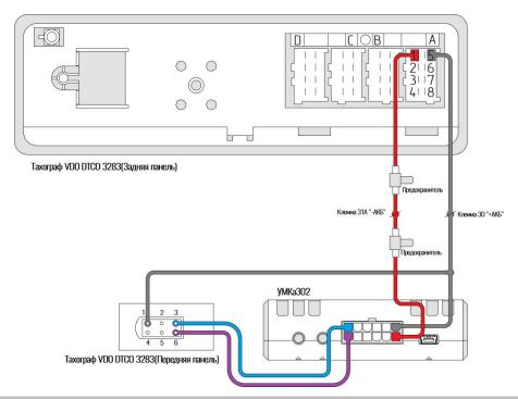
RS-232 line TX of the tracker UMKa-302 on contact 3 of tachograph front side adapter.
