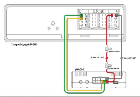
RS-485 line A of the tracker UMKa-302 on contact D1 of tachograph.
