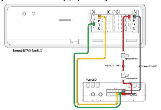
RS-485 line A of the tracker UMKa-302 on D3 tachograph contact.
