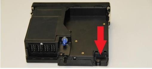
RS-232 line TxD of the tracker UMKa-302 on contact RS 232 RX (9).
