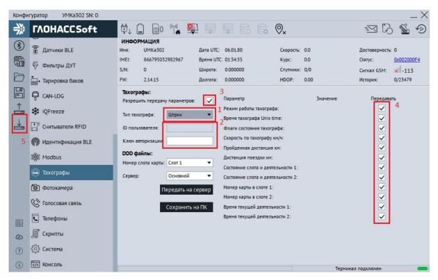
In the dropdown menu "Tachograph type" (1) you need to choose the type of connected tachograph. If neccessary, fill in the fields "User ID" and "Authorization key" (2). In case these parameters fields are left unfilled, factory values for corresponding type of tachographs are used.
